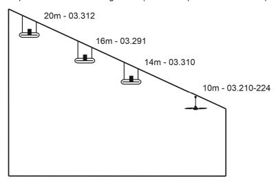
Even in halls that are higher than the maximum throw of the fans, perfect destratification down to the floor is possible. To do this, some of the fans are installed at the highest point and some of the fans are installed lower. If ceiling installation at different levels is not possible, you can install fans 03.291 or 03.310 at the side wall in slant position.
