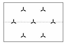
Important: You should always install some ceiling fans at the highest position of the room, to be sure no warmer air remains under the ceiling.
