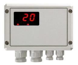
The controller recirculation hot air for an appropriate control of the fans. The device records the temperature near the floor and the ceiling with two temperature sensors in order to switch on or off the recirculation equipment (speed controller and fans).
