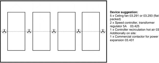
2 x Speed controller, transformer regulator 5A 03.425 1 x Controller recirculation hot air 03.431 Additionally on site: 1 x Commercial contactor for power expansion 03.431
